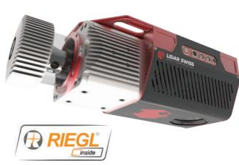
LS Micro Vux LR is the next generation LIDAR solution, a product suitable for both corridor and area mapping. Based on the Riegl VUX-1LR, survey grade FOG IMU, and including a 50mp RGB calibrated camera fully integrated. It can be operated at higher altitudes and covers more area on either manned, unmanned platforms or for mobile mapping.
